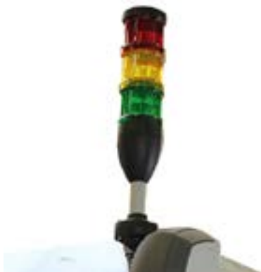
Machine status light
