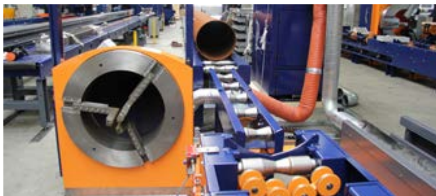
Transversal diabolo roller conveyor in position of the main drive (1200 version)
