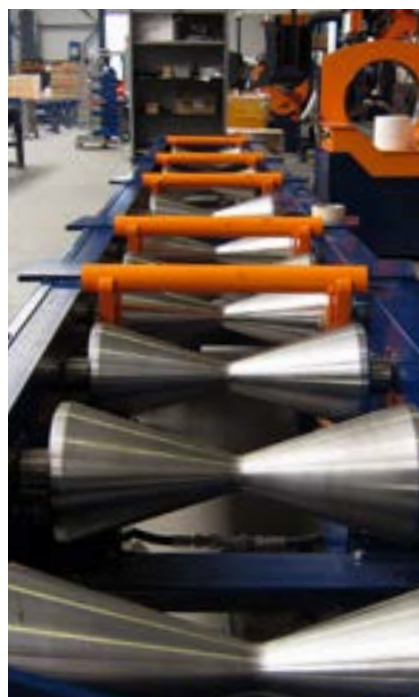
Diabolo rollers of the infeed table
