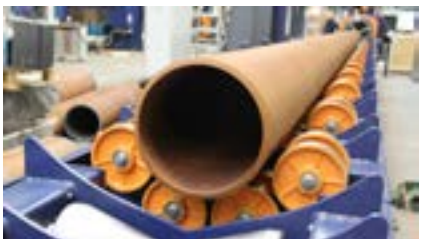
Resting on pipe support for rotation
