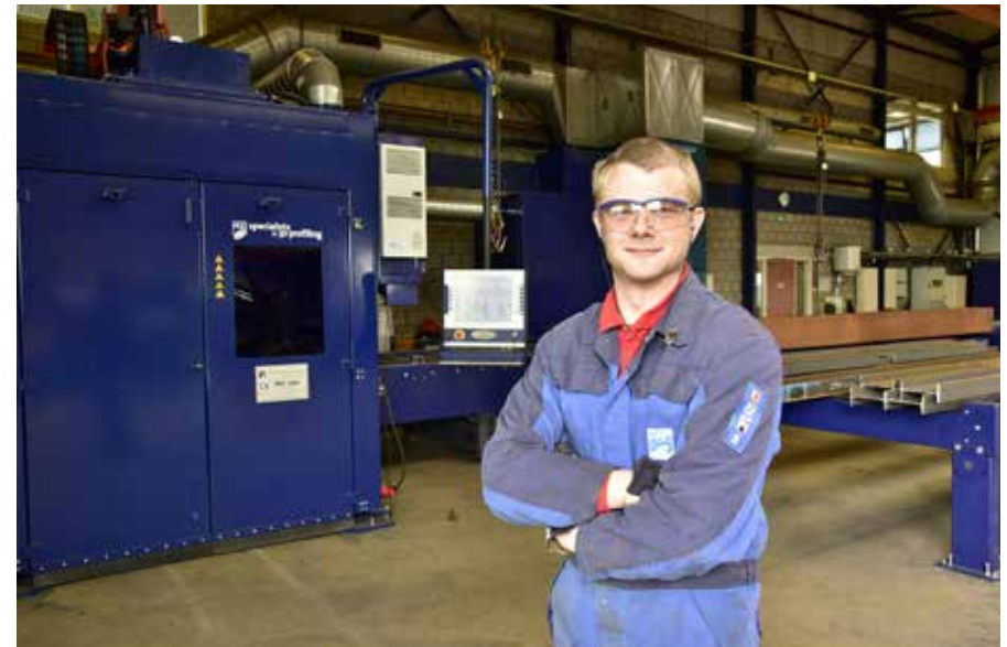
Operator in front of the closed of cutting cell and outfeed conveyor.
