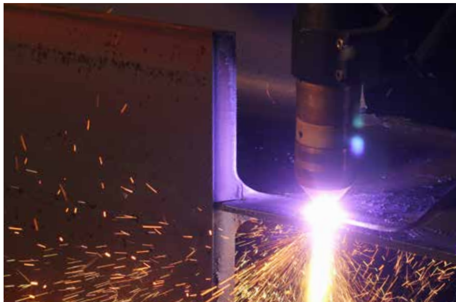
A plasma torch cutting through the web of a beam profile.
