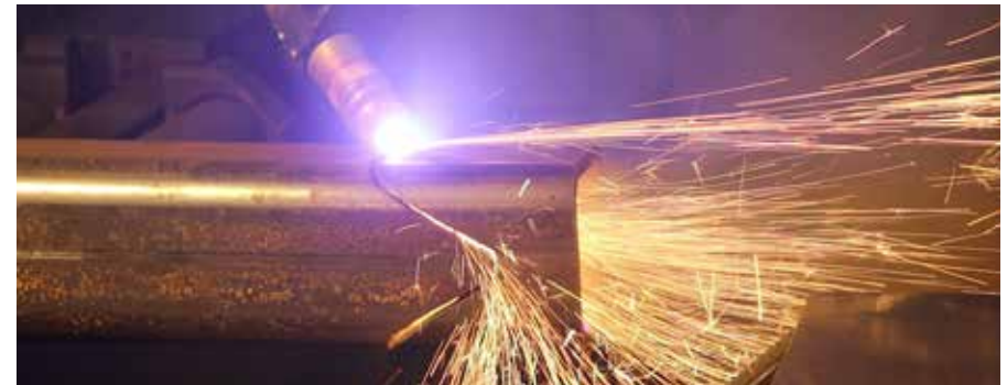
3D coping over the box-section corners
