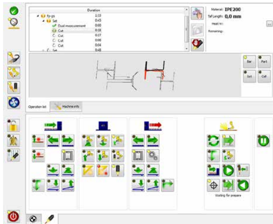
Operator GUI optimized for a touch screen. This screen is used during the cutting process.
