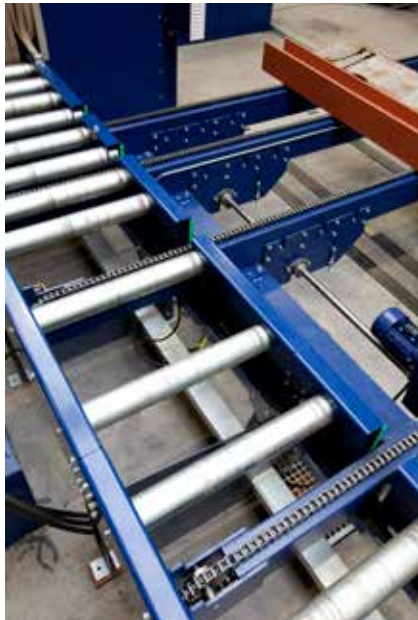
Infeed storage chains and infeed conveyor
