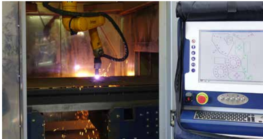
Plate cutting with cutting preview on the remote control.
