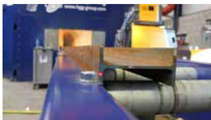
Length measurement laser on profile.
